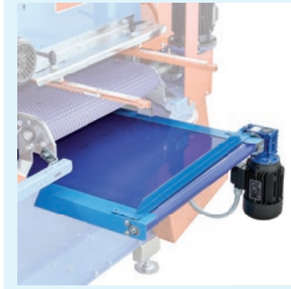
53 Belt system for the exceeding soil recycle.
